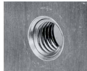
4. Remove tang from insert. You now have a permanently repaired thread.
