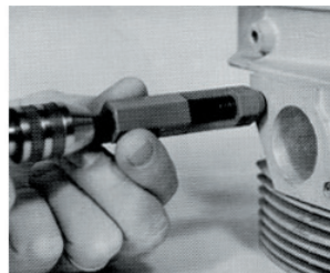
3. Install new Perma-Coil® insert. (Prewinding tool shown is used for fine thread applications only)
