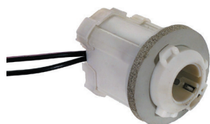
F22321 Socket Pigtail (2) 7" leads 18 ga. black and purple Ford trucks and Bronco '80-'90 for use w/ 1156 bulbs White Housing
